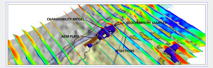
Geological map with IP section integrated with chargeability 3D model, EM plate model and the Zn geochemistry.
